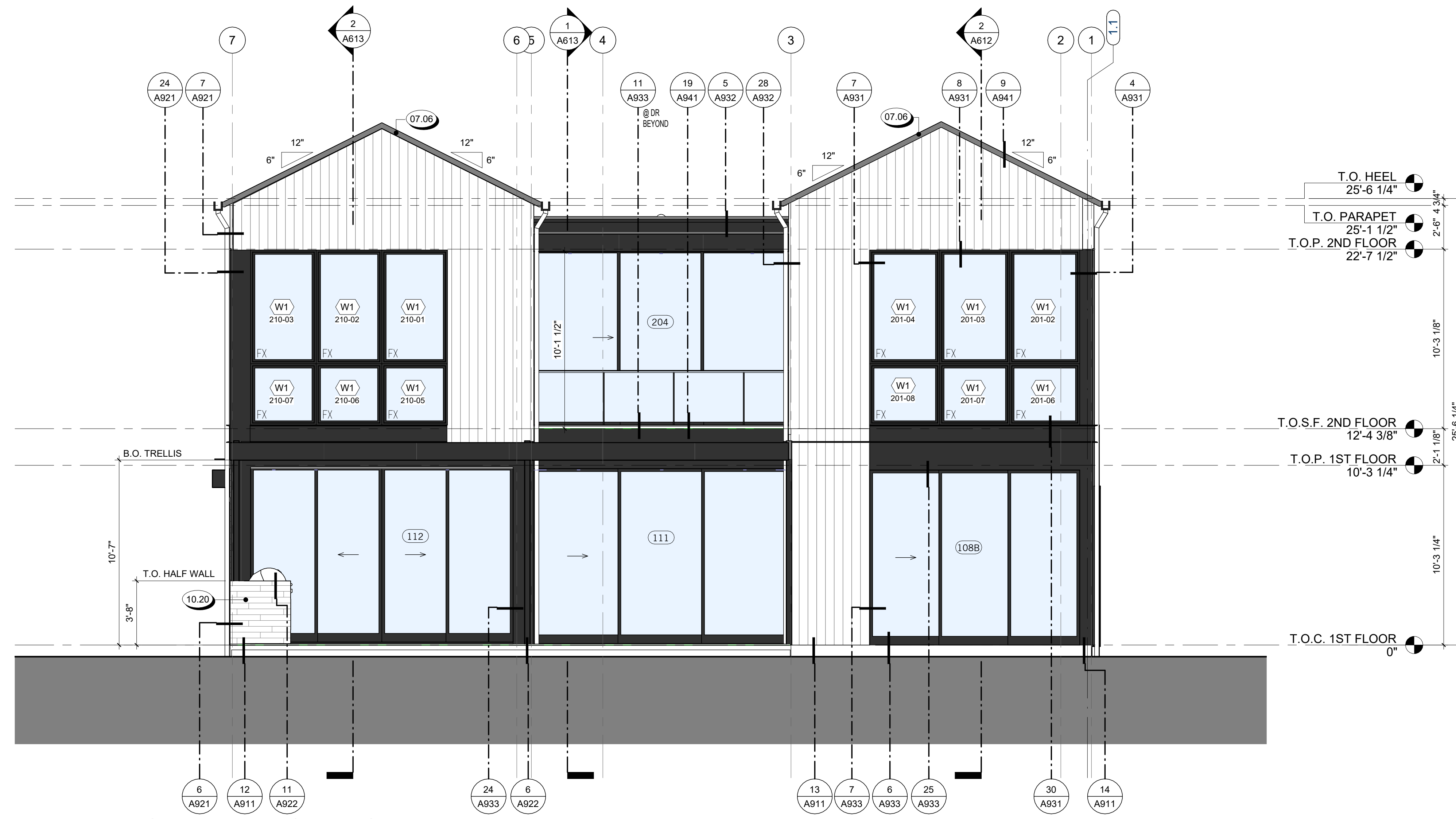
1 EXTERIOR ELEVATION - NORTH 1/4" = 1'-0"
