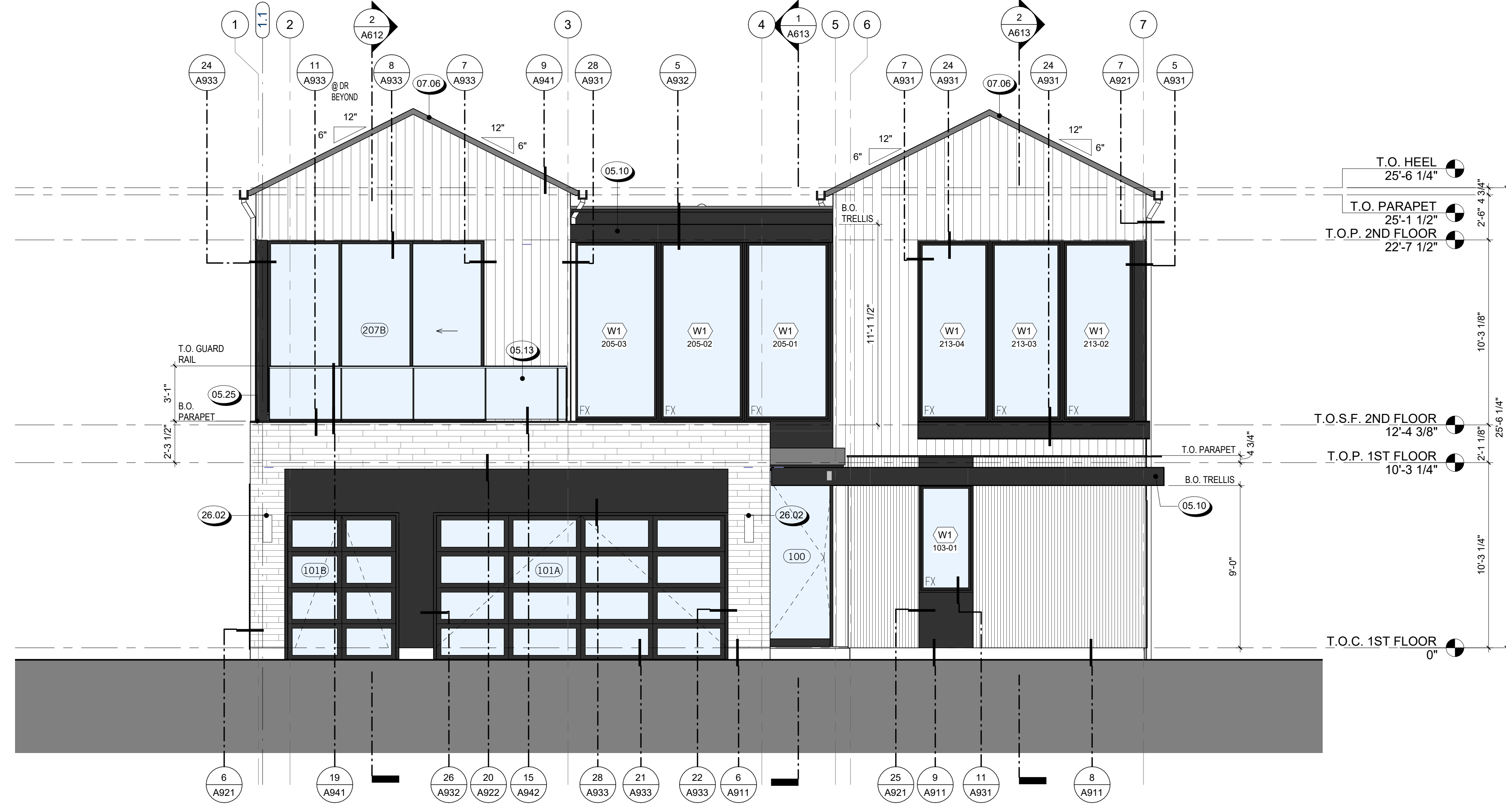
2 EXTERIOR ELEVATION - SOUTH 1/4" = 1'-0"
