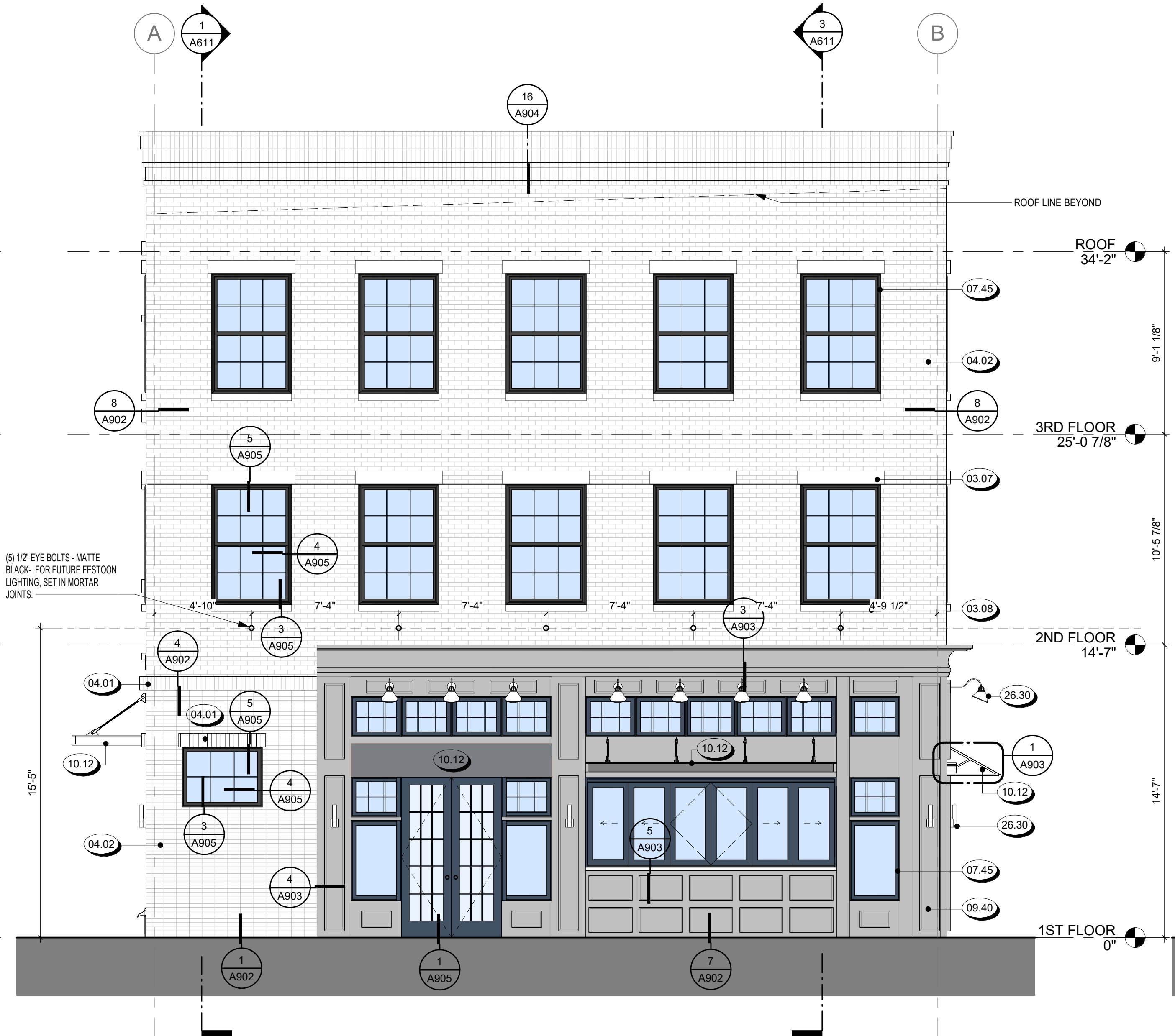
3 EXTERIOR ELEVATION - SOUTH 1/4" = 1'-0"
