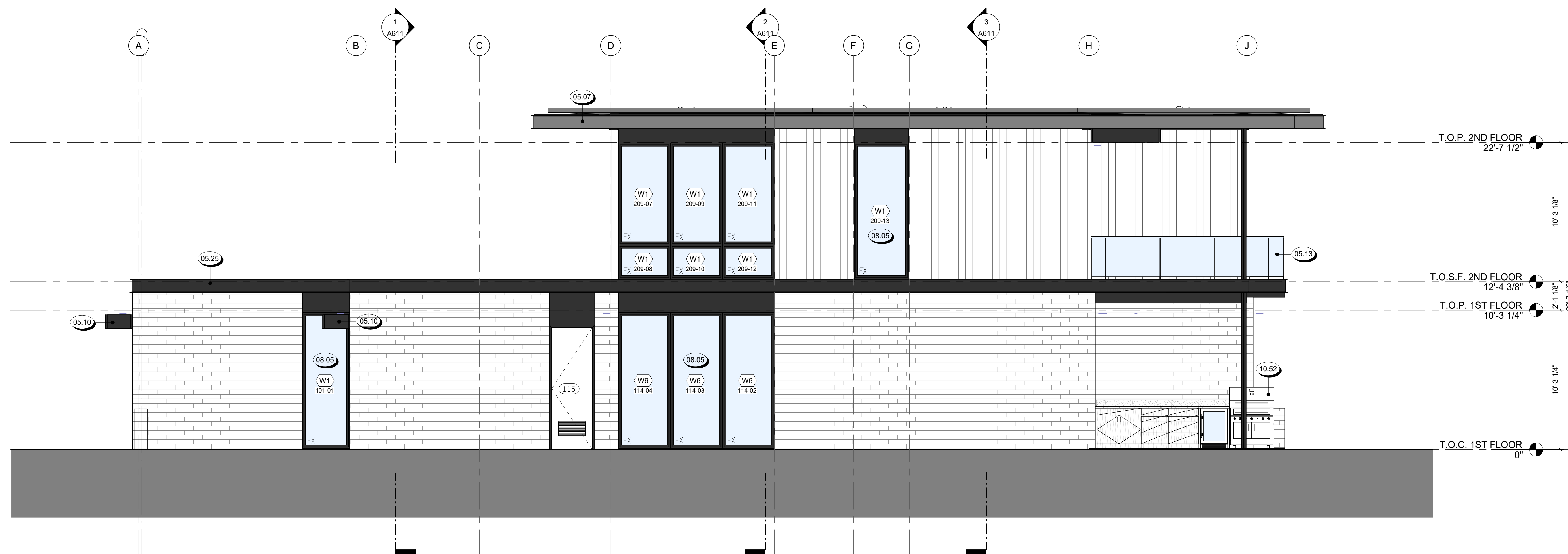
1 EXTERIOR ELEVATION - SOUTH 1/4" = 1'-0"
