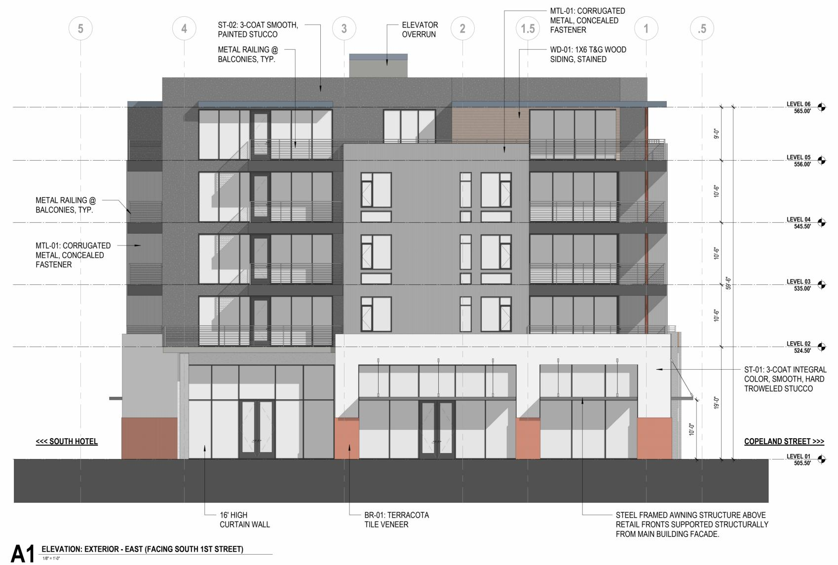
**ELEVATIONS GENERAL NOTES** storybuilt. 1. PLACEHOLDER 900 S. 1st St., Suite 110 Austin, Texas 78704 512.289.1313 storybuilt.com KEY PLAN NOT FOR CONSTRUCTION These documents are incomplete, and are released for interim review only and are not intended for regulatory approval, permit, or construction purposes.
