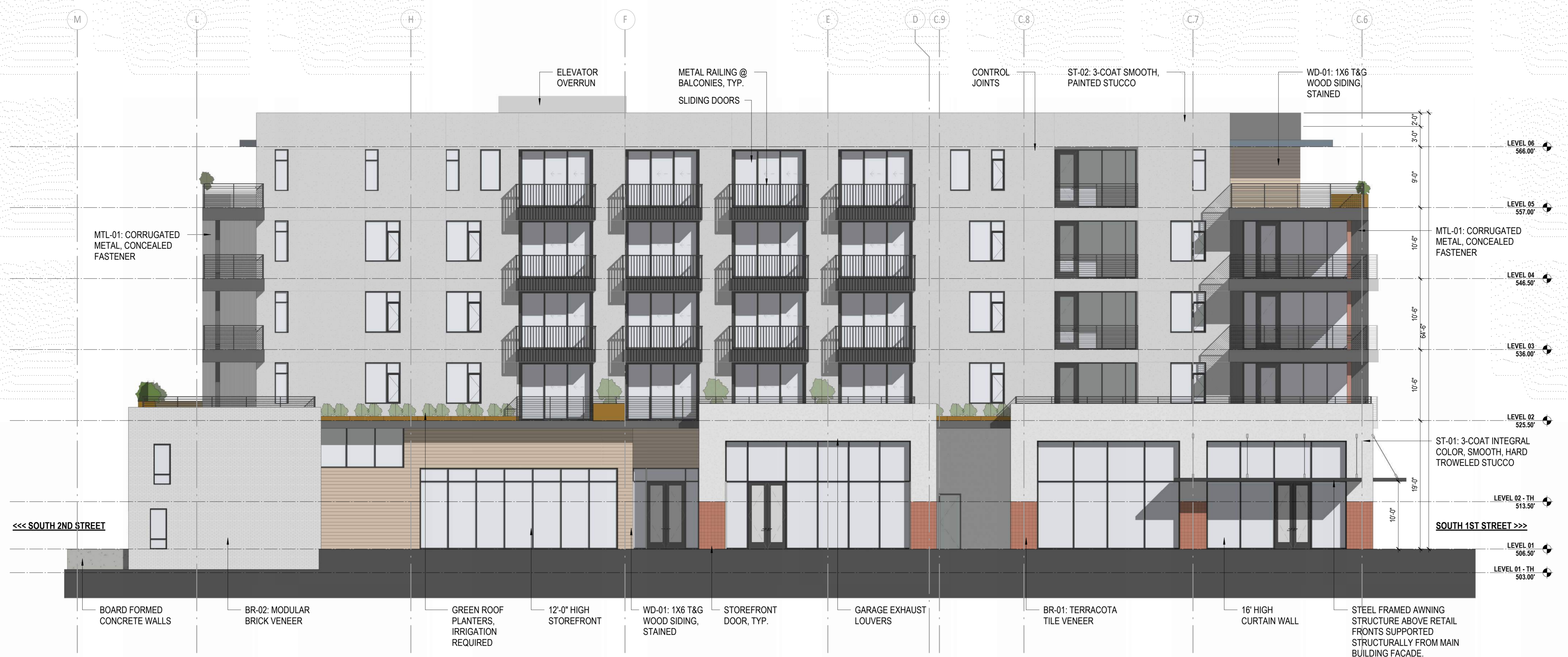
2 ELEVATION- EXTERIOR - SOUTH (FACING COPELAND STREET) 1/8" = 1'-0"
