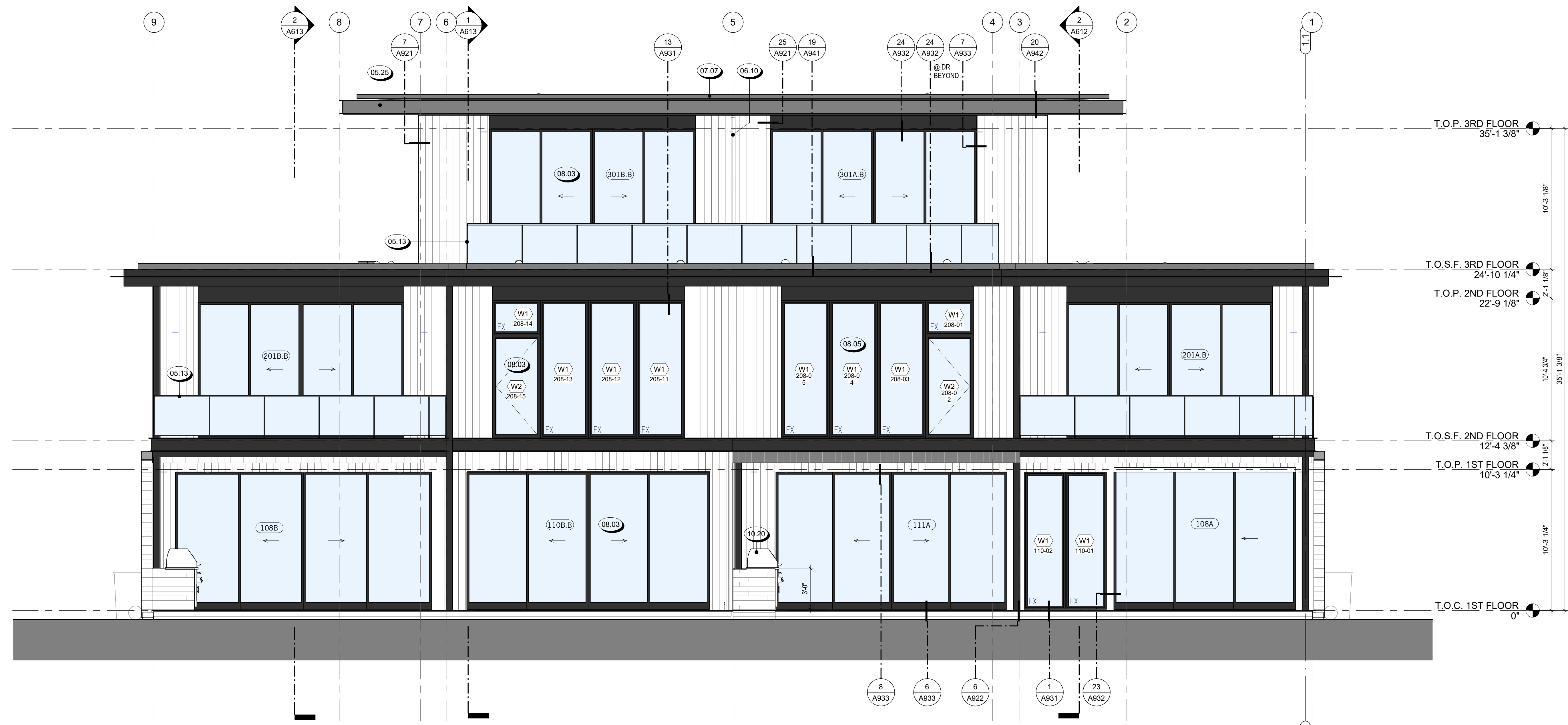
1 EXTERIOR ELEVATION - EAST 1/4" = 1'-0"
